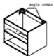
5. Install 1 angle codes on 20860-3 panel hole to hole fixing by 4x6x12 screws
