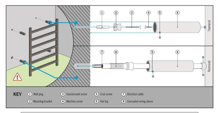
**WARNING:** This is a 12Volt heated towel rail and MUST be wired to a transformer (supplied). Connecting directly to the mains power supply will cause irreparable damage to the element and the element cannot be replaced.
