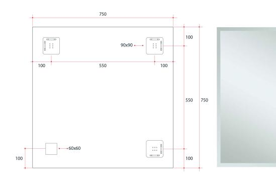
Note: All dimensions are in millimetres (mm)
