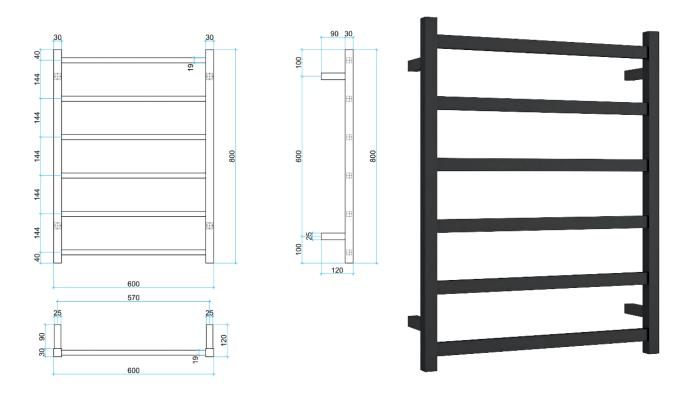
This rail has Multiflex wiring which means that there is a connection point on both the left and right hand side of the rail and the lead can be connected to either side. Being a dry electric element rail, this can be mounted either way up meaning the wiring can be from any of the four mounting points.
