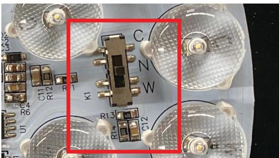
Choose colour temperature by flicking the switch in the LED (See Fg.10)
