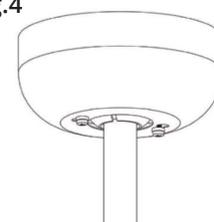
After wiring is completed, attach the canopy to the hanger bracket by pushing upwards and twisting anti-clockwise. Tighten screws and ensure canopy is not touching the ball joint. (See Fg.4)
