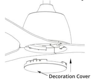
**To install:** Align face plate with the blade gap before pressing.
