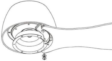
The screw installed on the upper housing must align at the gap as shown. (See Fg.5)
