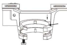
Secure the hanger bracket to ceiling beam or a suitable piece of timber inserted between the ceiling beams using the two long screws supplied with the package. (See Fg.1)
