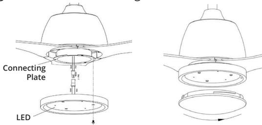
**To install:** Remove the screw from the connecting plate. Plug the wire into the light kit mounting hole. Align the thread with connecting plate before tighten the screw.
