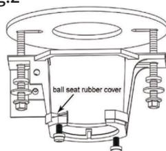
Place circular shockproof gasket above the hanger bracket. Align the bracket and screw the hanger bracket to the ceiling tightly. (See Fg.2)
