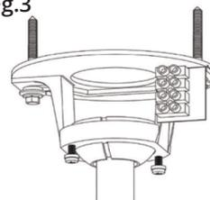
Place fan into hanger bracket and align Ball Joint Slot with hanger bracket as illustrated. (See Fg.3)
