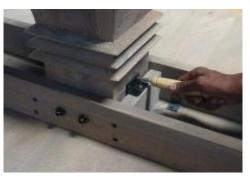
**STEP- 03** Place the metal angle near the leg as shown in picture. Match the hole of angle with hole of insert. Tighten the metal angle with pen head allen bolt with washer by allen key. Don't tighten fully, tighten the metal angle with leg by screwing in given wooden screw by screw driver. Tighten allen bolt fully.
