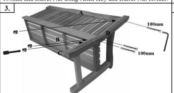
Fix Back Rest  $\underline{\mathbf{A}}$  to Seat  $\underline{\mathbf{B}}$  and Side  $\underline{\mathbf{D}}$  (Left) with 3pcs Screw M6 x 100mm and Barrel Nut using Allen Key and Barrel Nut Holder.
