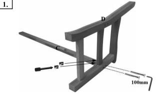
Fix Side  $\underline{\mathbf{D}}$  (Left) to Seat Support  $\underline{\mathbf{C}}$  with 2pcs Screw M6 x 100mm and Barrel Nut using Allen Key and Barrel Nut Holder.
