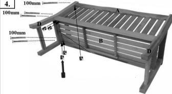
Fix Side  $\underline{\mathbf{D}}$  (Right) to Back Rest  $\underline{\mathbf{A}}$  and Seat Support  $\underline{\mathbf{C}}$  with 5pcs Screw M6 x 100mm and Barrel Nut using Allen Key and Barrel Nut Holder.
