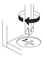
Turn cam lock clockwise to tighten.
