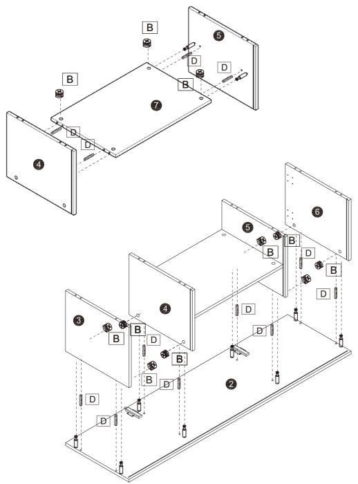
Assemble the parts in the manner shown. Ensure that each part is installed in the correct position. Use B,D screws for fixing.
