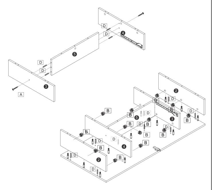
Use  $15 \times 10$ mm,  $6 \times 30$ mm, and  $M4 \times 30$ mm screws for fixing. Different positions may require different screws, so please check carefully before installation.
