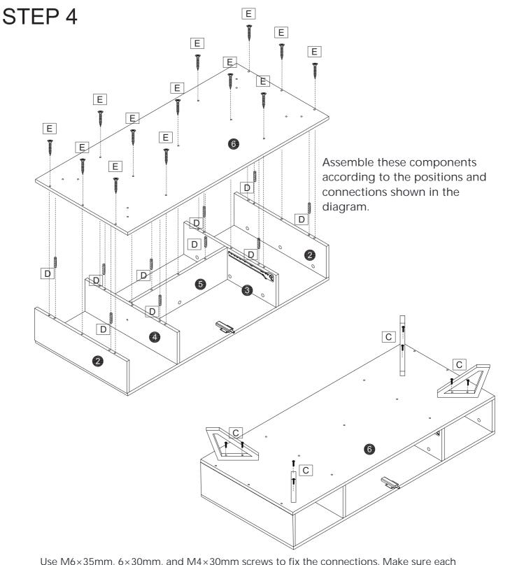
Use M6 $\times$ 35mm, 6 $\times$ 30mm, and M4 $\times$ 30mm screws to fix the connections. Make sure each screw is tightened properly to ensure the overall stability.
