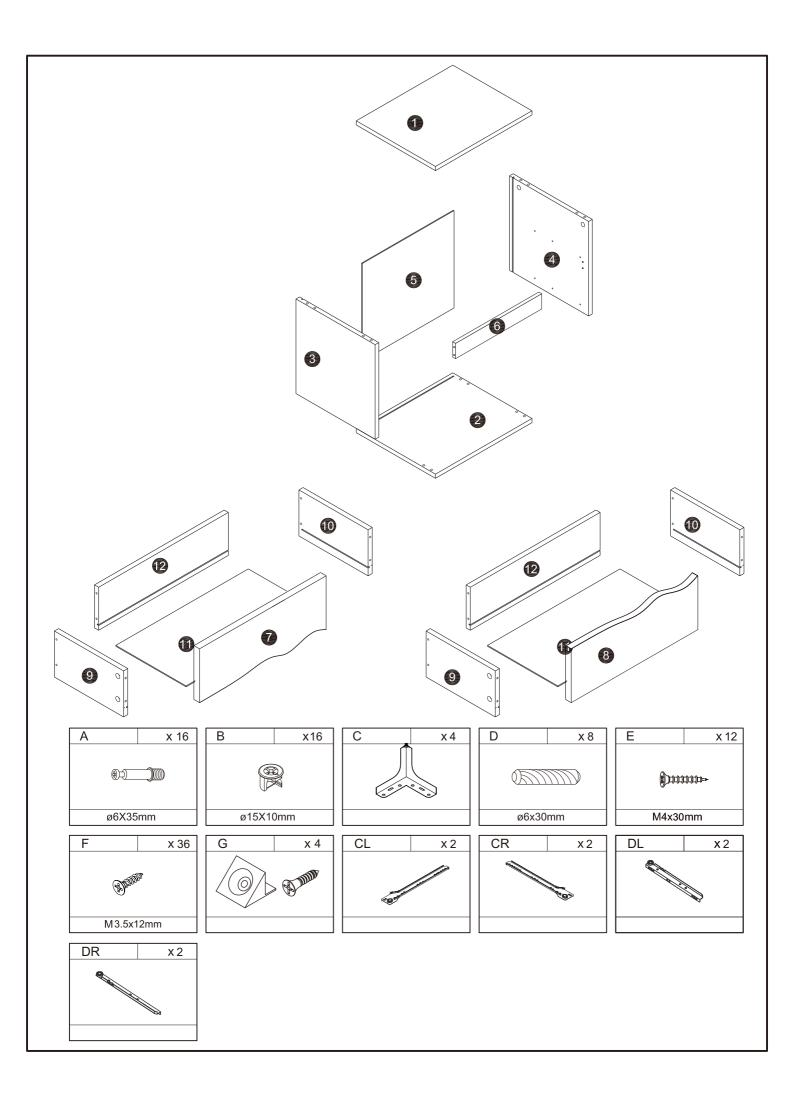
Attach CL and CR to the left and right sides of the base frame.
