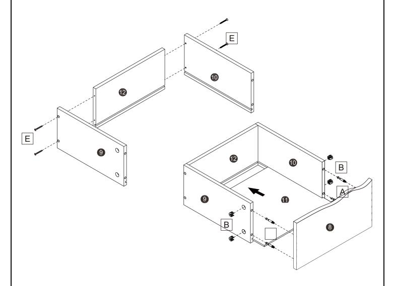
Use A,B and E screws to secure the connections. Different positions may require different screws,so please check carefully before installtion.
