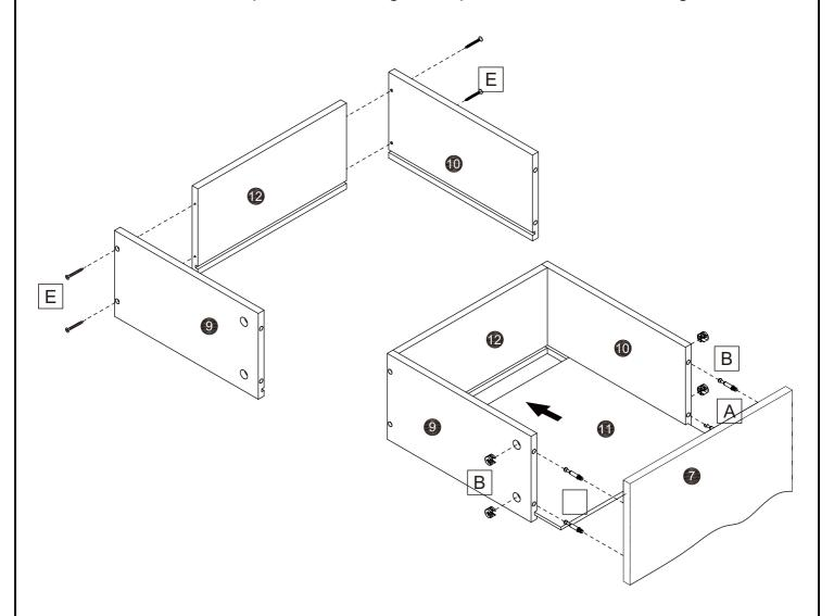
Use A,B and E screws to secure the connections. Different positions may require different screws, so please check carefully before installation.
