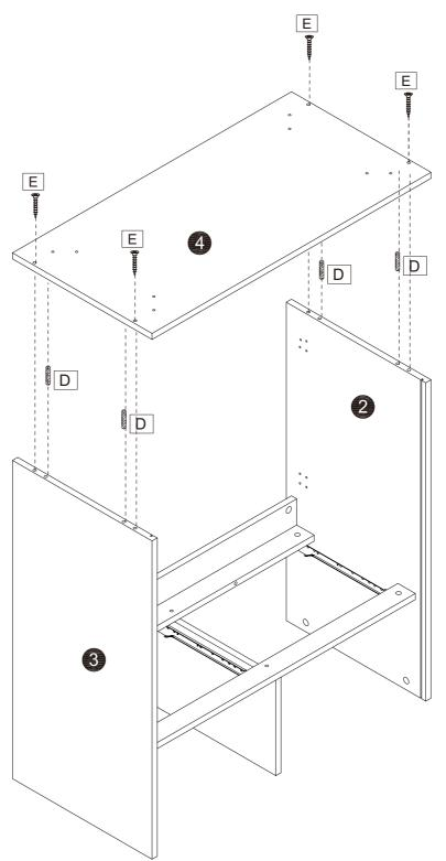
Assemble D and E according to the diagram. Connect them firmly to form the required structure. Use D,E screws to secure the connections.
