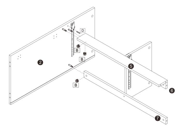
Assemble the components shown in the diagram. Layer them as needed to form the structure. Use B<sub>1</sub>D screws to secure the connections.
