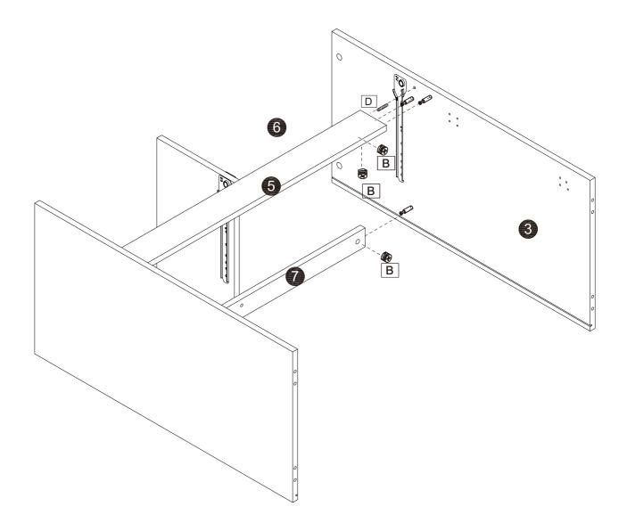
Assemble the parts in the manner shown. Ensure that each part is installed in the correct position. Use B,D screws to secure the connections.
