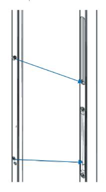
**B** Slide the drop side up to the top point, then gently pull the head out of the round plastic mechanism.
