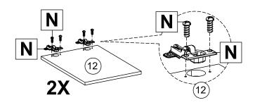
Step 15 Attach 2 x Door (12) to case assembly as shown.
