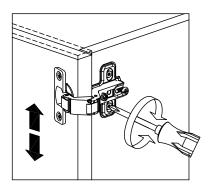
To move doors up or down: loosen or tighten the screws on the hinge plate, as shown.
