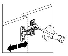
To move doors in or out: loosen or tighten the screws on the hinge plate, as shown.
