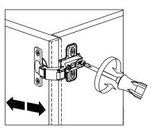
To move doors in or out: loosen or tighten the screws on the hinge plate, as shown.
