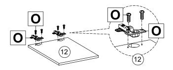
Step 18 Attach Door (12) to case assembly as shown.
