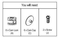
Attach Left Panel (3) and Right Panel (4) to case assembly using 6 x cam lock (A) as shown, Use a screwdriver to turn the Cam lock clockwise to lock. Paste 6 x Cam Cap (C) as shown.
