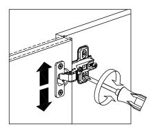
To move doors up or down: loosen or tighten the screws on the hinge plate, as shown.
