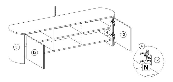
Step 16 The doors might out of alignment after the transportation. If adjustment is necessary, please follow the steps below:
