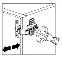
To move doors left or right: loosen or tighten the screws on the hinge plate, as shown.
