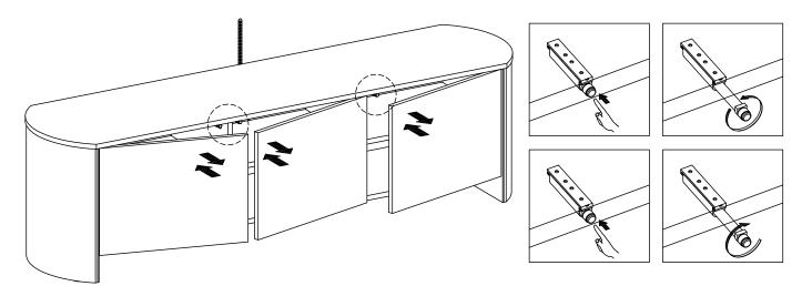
After transportation, the push to open latches may need to be adjusted if it does not work well.
