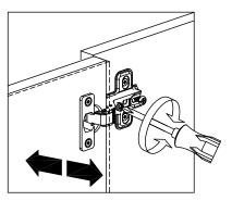
To move doors left or right: loosen or tighten the screws on the hinge plate, as shown.
