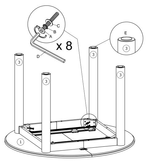
Attach 2 x Legs (2) to Body (1) using 4 x Bolts (B), 4 x Spring Washers (C) and 4 x Washers (D). Tighten the bolts with Allen Key (E) .
