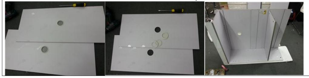
5, the fifth step is to install the other side panel and to tight all screws by using part A & K. It will use a lot of the big round buckles. DO NOT miss the holes underneath and those holes of fixed shelf.
