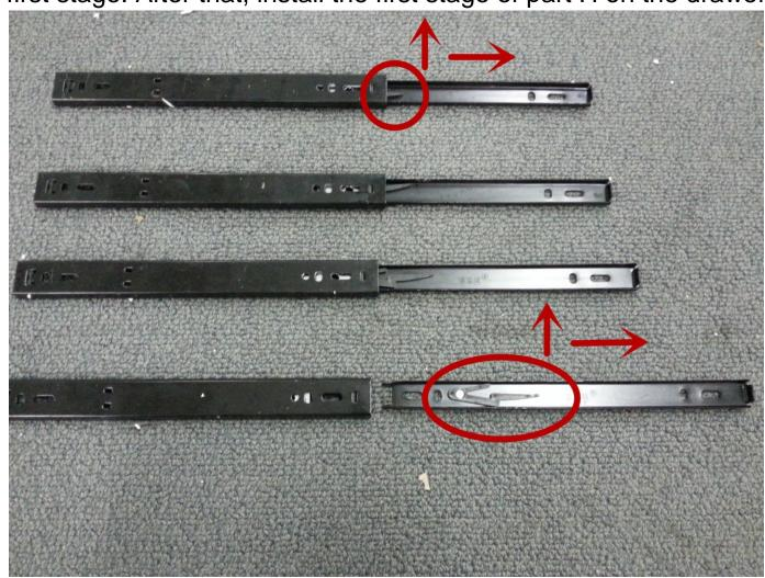
9, The ninth step is to install the rest of Part H on the side panels and drawer support. Then put the drawers into the tracks. If your first attempt is unsuccessful, you can repeat the eighth step, remove the drawers and adjust part H and try again.
