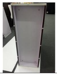
6, the sixth step is to install drawer support panel by using part A, there is a small hole on the side of the small panel, which should face to the back. Tight all the parts A & K.
