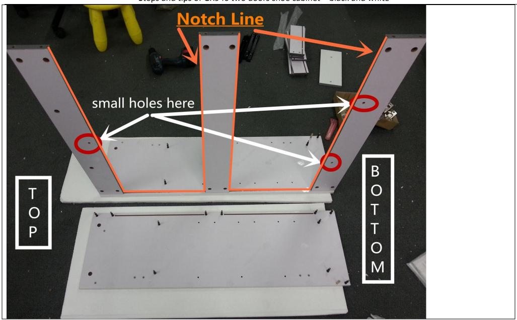
3, the third step is assembling the fixed shelf and the bottom. Their holes should face to the bottom.
