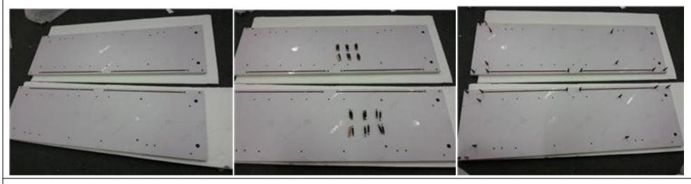
2, the second step is to installing three back bars. Pay attention to three different back bars, their holes should face backward.
